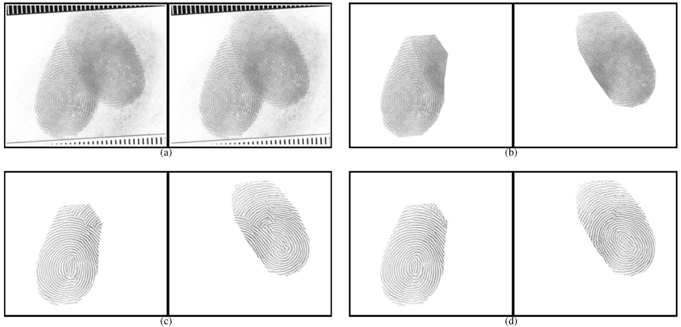
Fig. 12. Query fingerprints of four groups of matching experiments. (a) Overlapped fingerprints (i.e., no separation); (b) overlapped fingerprints separated by mask images; (c) component fingerprints separated by our previous method [8]; (d) component fingerprints separated by the proposed method.
